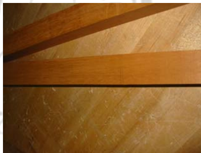
Jim Stevens and Tony Albano brought in the legs and described how they tapered the legs on a planer table
