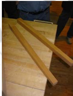
Jim Stevens and Tony Albano brought in the legs and described how they tapered the legs on a planer table
