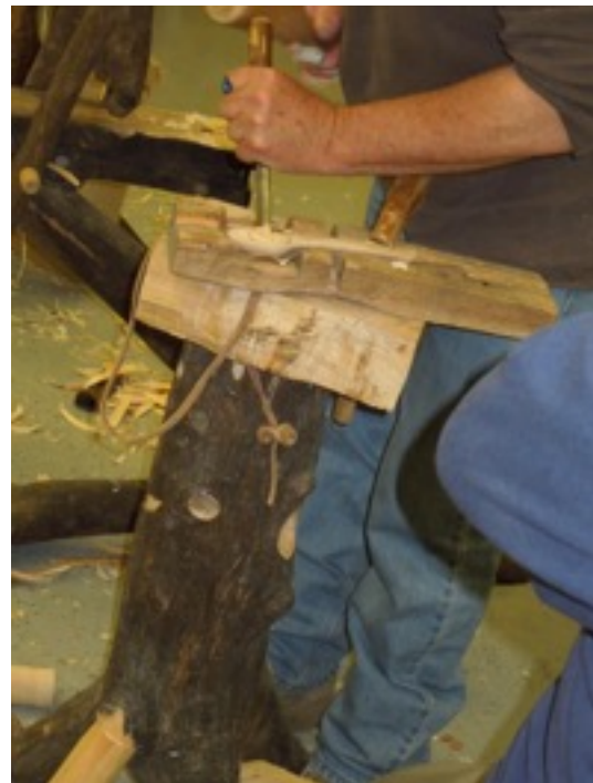
Shaping a spoon mounted in a jig.
